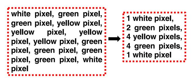
The description of the Mario image, for example, can be compressed by describing its pixels as shown in the second red box.
