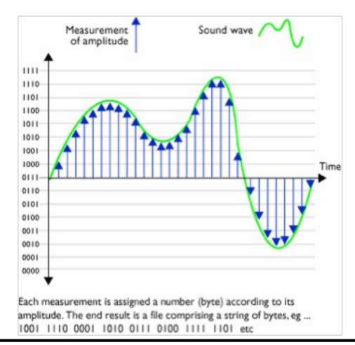
These points correspond, in the Cartesian plane, to precise coordinates, whose numerical value is used as coding of the "sampled" sound. The encoded sequence of the samples constitutes the encoding of the entire sound data represented by the wave.
