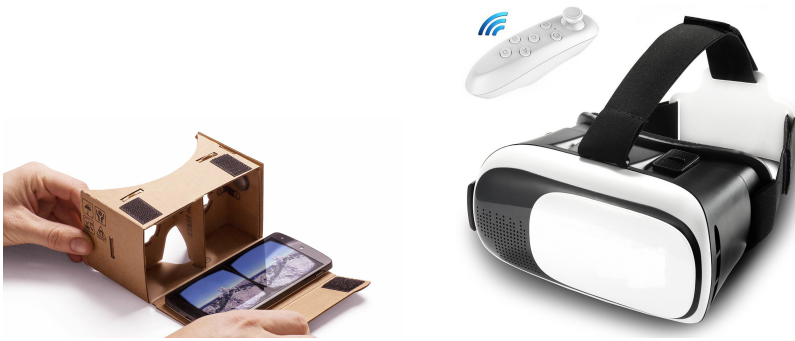
Fig. 1: The original Google Cardboard VR visor and a plastic variant
