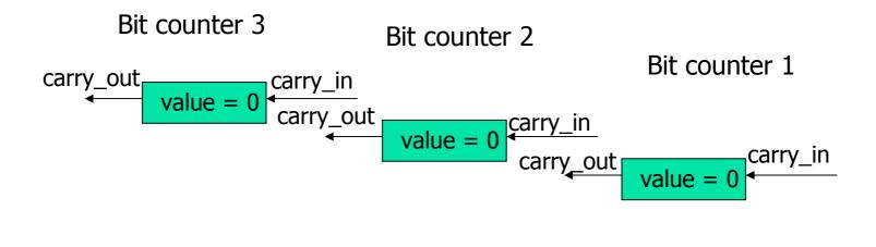
The first counter has input 1, while the other two have as input the carry\_out of the previous counter
