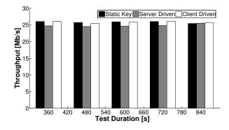
Figure 9: TCP throughput measured in the full-mesh network scenario for different key delivering protocols.
