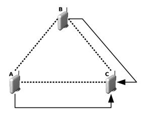
Figure 8: Full-Mesh Topology. A data transfer is performed between nodes A and C. Although C also acts as Key Server, the connection among the three nodes remain available.
