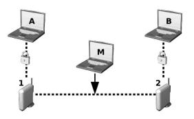
Figure 1: Alice and Bob exchange data through the wireless mesh network. Mallory will be able to eavesdrop their data, unless a security system is implemented to protect the backbone link.
