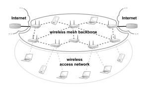
Figure 6: MobiMESH architecture.
