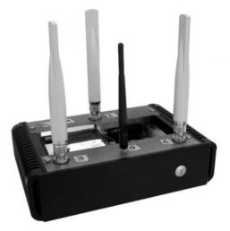
Figure 7: Multi-radio MobiMESH router.
