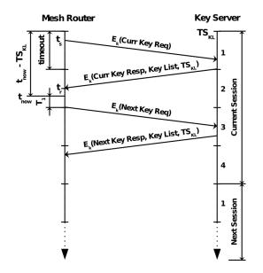
Figure 4: Server Driven Protocol. Since the first request has taken a time greater than *timeout*, the mesh router sends the successive request when it sets the third key.
