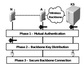
Figure 2: Phases of the connection process performed by a new mesh router (node N). The depicted keys are used to encrypt the backbone traffic.
