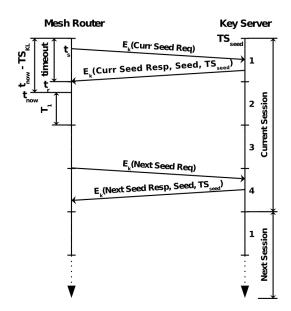
Figure 5: Client Driven Protocol. Since the first request has taken a time smaller than *timeout*, the mesh router sends the successive request when it sets the fourth key.
