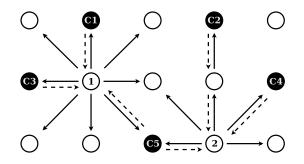
Fig. 2. Distributed Proactive Request Protocol. A (5,3) threshold scheme is adopted in this example WMN, where black and white circles represent, respectively, core and generic nodes. Solid lines represent requests, while dashed lines represent core node responses.
