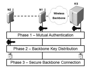
Fig. 1. Centralized security architecture: phases of the connection process performed by a new mesh router (node  $N_2$ ). The depicted keys are used to encrypt backbone traffic.
