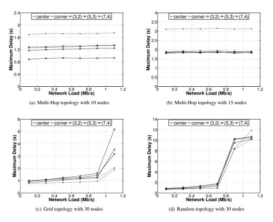
Fig. 7. Maximum Delay (in seconds) measured in the Multi-Hop, Grid and Random topologies.
